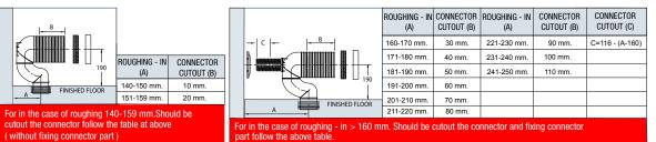
Fixing bracket & S-trap installation
