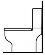
The pan and cistern are joined together so you can't see the flush pipe. These toilets only come in S Trap installs where the pipe comes out of the ground, and the pipe must be in the exact location or within 20mm for installation to be possible.
