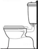
The cistern and pan are connected by a flush pipe. These toilets due to the connecting flush pipe are most flexible for install.
